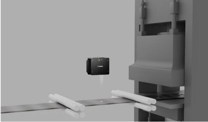
This sensor can measure coil feed amount correctly without contacting the material. This prevented defective products and mold damage, reducing fix costs and improved productivity.
