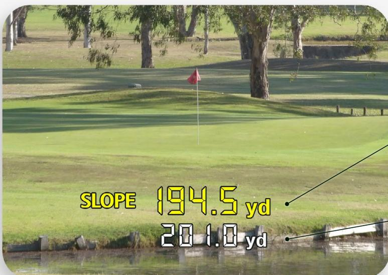
Effective distance that the ball must travel (horizontal distance  $\pm$  height) with Slope Mode **ON**
